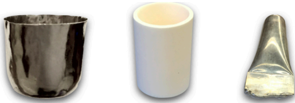
Figure I.2: Reaction vessels for flux reactions. Platinum crucible (left), alumina crucible (middle), silver tube (right).
